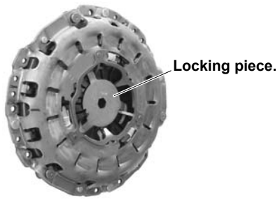
Fig. 28: Clutch-centring pin in clutch disc.
