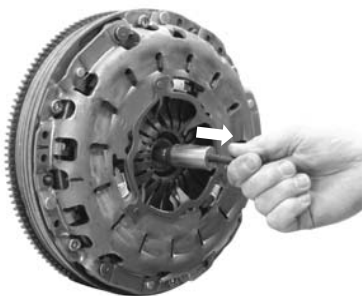
Fig. 31: Remove clutch-centring pin.
