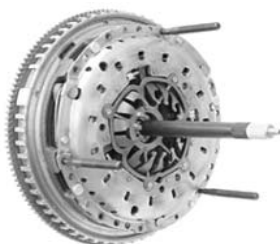
Fig. 10: Remove clutch aligner and threaded bolts.
