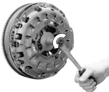
Fig. 31: Remove clutch-centring pin.
