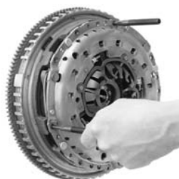
Fig. 11: Remove clutch pressure plate and clutch disc.
