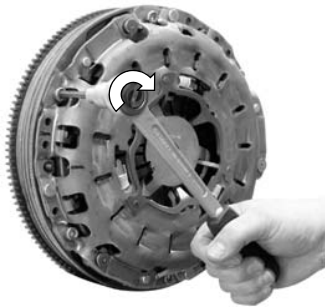
Fig. 30: Unscrew locking piece.
