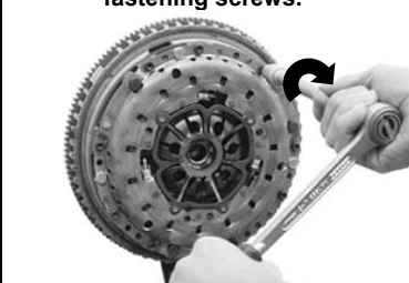
Fig. 26: Screw in and tighten clutch pressure plate fastening screws.
