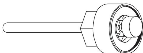
2. THE TOOL ALLOWS QUICK AND EASY REPLACEMENT OF THE INNER BALL-JOINT ON THE STEERING RACK. REMOVAL OF THE RACK FROM THE BULKHEAD IS NOT NECESSARY.
