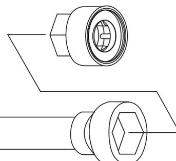
3. FIT THE APPROPRIATE LOCKING TOOL TO THE EXPOSED USING THE SPECIAL SOCKET UNDO THE BALL JOINT OF THE RACK STEERING RACK SIMULTANEOUS LOCKING THE RACK USING THE CHOSEN LOCKING TOOL. AFTER THE REMOVAL OF THE BALL JOINT IT IS NOW POSSIBLE TO REPLACE THE SEALING RING IN RACK HOUSING.
